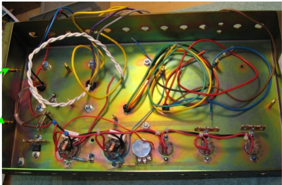
Heater wires carry AC and should be strung at least 1" or so above the tubes, and twisted or wrapped closely together:
