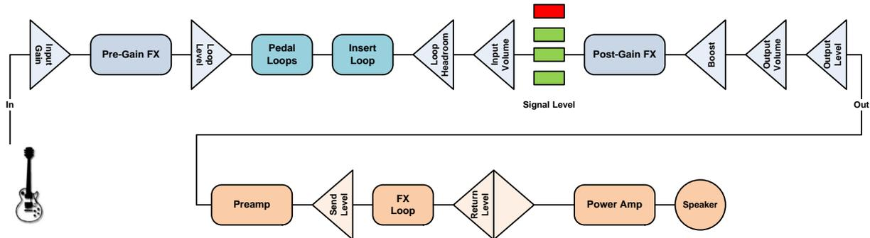
As you can see in the diagram above, the G-System can be placed between the guitar and amp such that all of the G-System features (loops, FX) are placed before the amp input. If you have an old combo amp or head that does not have a loop, this is your only option.
