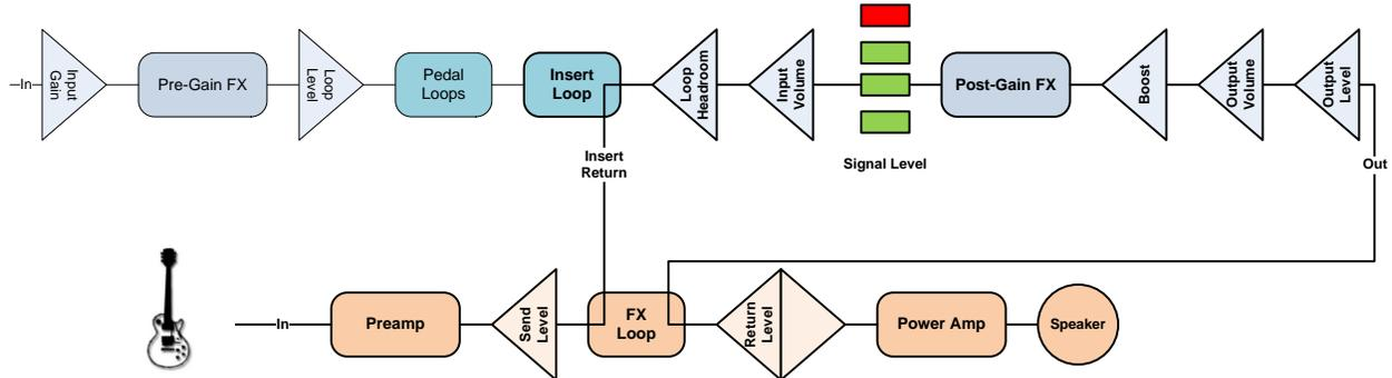
The diagram above shows the signal path of the G-System when we bypass the front end and put just the back end in the amp's FX loop. Notice that nothing from the G-System input to the insert send is in the signal path – so any issues we encounter in this configuration can't originate in these components. Also, if we are clever and patient about when we hook up the three cables involved, we can quickly isolate and (often) solve problems introduced at each connection point.
