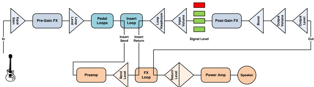
In most cases, this is the optimal way to hook up the G-System to your amp. This is what the G-System engineers really intended. In this configuration, pre-gain FX and the pedal loops come before the preamp, post-gain FX and pedals go in the loop. Component locations are “optimized” according to what most people see as the best way to connect amp and FX.
