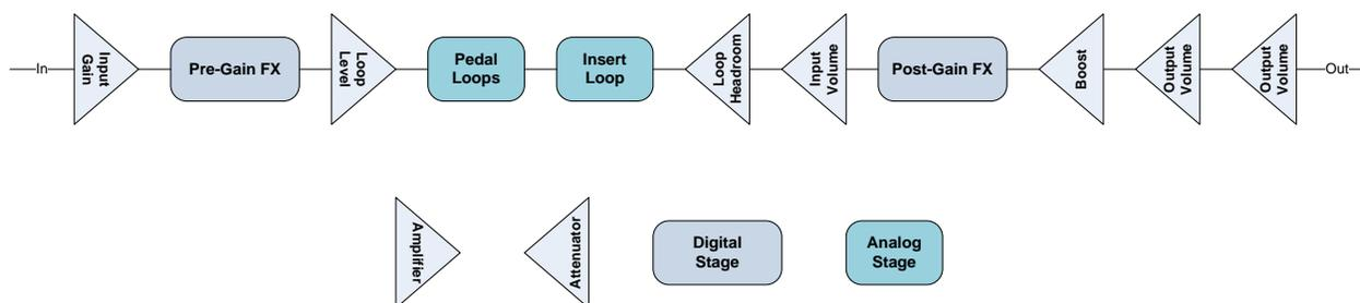
You'd probably be surprised to notice that there are only two spots on the G-System that have any kind of amplifier, just before and after the pre-gain FX. All the other signal level adjustments are about if and how much you attenuate the signal (make it quieter). They have no mechanism for amplifying the signal. This will become very important later.
